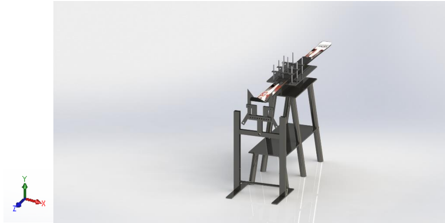
Figure 3 Rig design with additional table structure.
